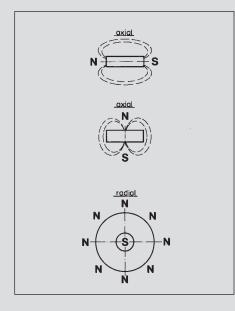
The preferred direction is achieved by subjecting the magnetic powder to a strong external magnetic field (coil) during the pressing process. As magnets have no preferred direction, the magnetisation direction and type can be freely selected. Mounting a magnetic switch system on ferromagnetic materials
